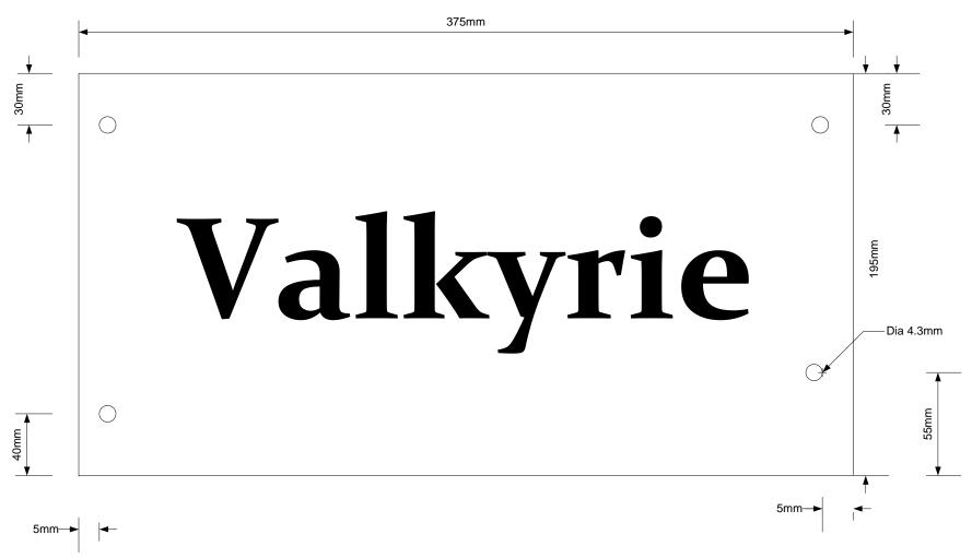
All measurement to the holes are to the centre of the hole. 4mm mounting bolts for the grill
